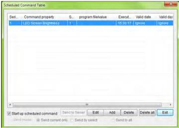
Start up scheduled command: select to enable Scheduled Command Send to Server: applied in Remote LED Screen Manager Online mode Note: Send to Server details, please refer to Page49 **Send current only**: send the **Scheduled Command Table** to the current selected led display
