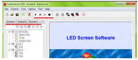
**Normal Display:** For No-Sending Card Mode Only. LedStudio capture the contents of **Screen Area** and send directly to receiving cards.
