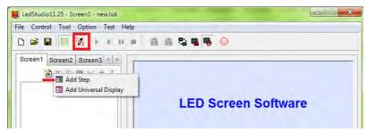
**Add Step**: Steps are played in order, from Step 1 to Step 2 to last Step then back to Step 1. It is Step1 to Step Last to Step1 circle loop play.
